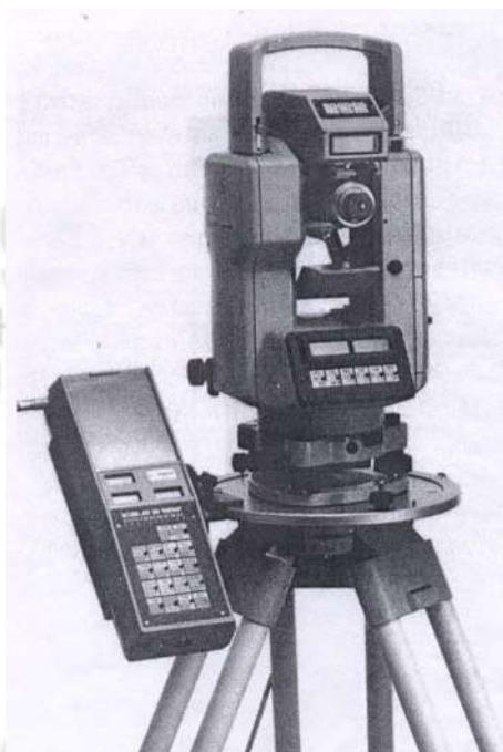
Figure 5.1 : An Electronic Theodolite with Data Collector
